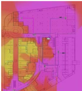
Figure 3: The level of radio field coverage inside the object (ground)
