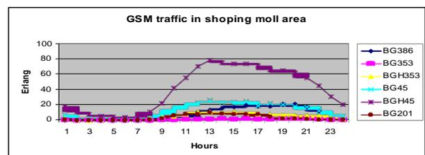
Figure 6: Total 24 hours traffic on GSM base stations
