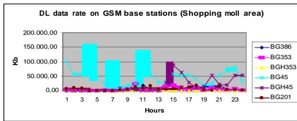
Figure 8: DL data rate on GSM base stations
