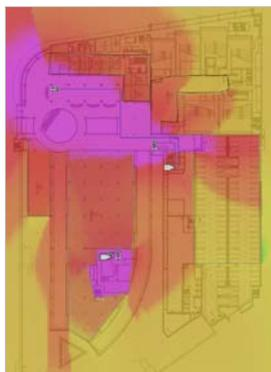
Figure 5: The level of radio field coverage inside the object (II floor)
