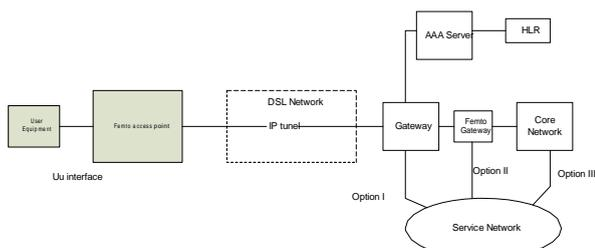
Figure 1: The block-scheme of femto cell solution
