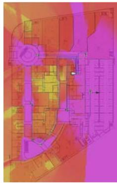
Figure 4: The level of radio field coverage inside the object (I floor)
