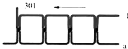
Figure 3. Lockstich type 301 ( 1- upper needle thread, a- lower thread-shuttle thread)
